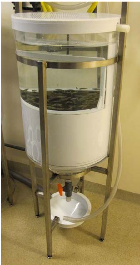
**Fig. 2** Zebrafish spawning vessel. More than 200 fish can be spawned simultaneously in the vessel, giving rise to  $\sim 10,000$  highly synchronized embryos in a short time period. With its slim design, the apparatus takes up a small footprint. (For color version of this figure, the reader is referred to the web version of this book.)
